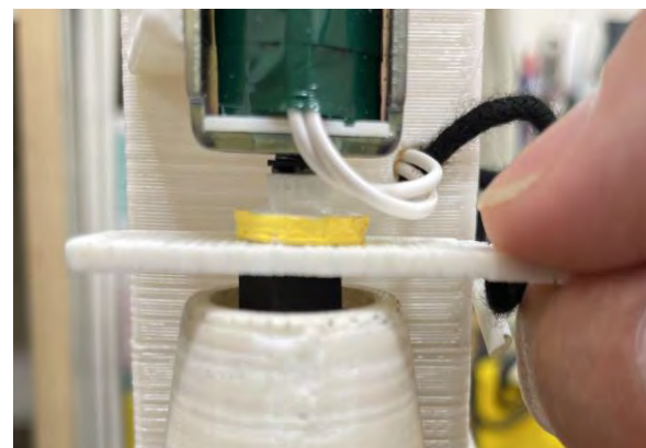
Figure 6 Spacing adjustment between solenoid and button
