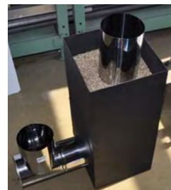
Figure 5. The final product of the rocket stove
