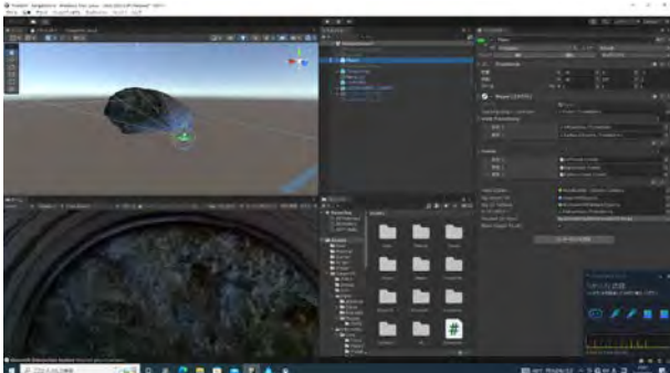
Photo 2 The 3D model around the tunnel face imported into the VR space of Unity.
