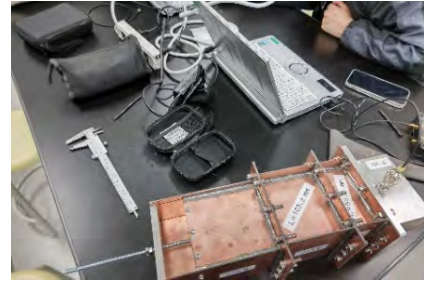
Figure 20. A photograph of impedance matching practice of a waveguide (bottom) in the GHz region using a NanoVNA (right) and its control PC.
