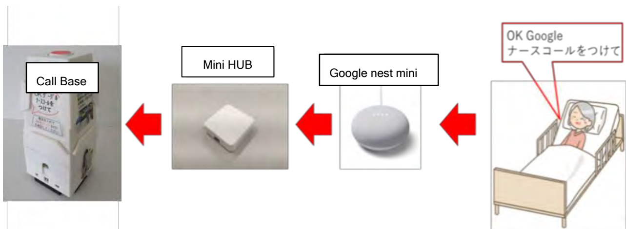
Figure 2 The equipments used and the flow of operations
