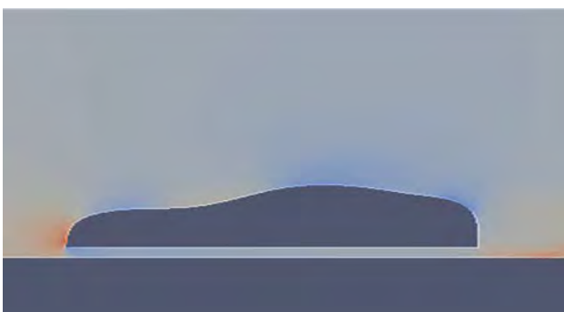
Figure 9 Flow pressure distribution in the center cross-section of the car body
