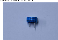
(b) A sample battery: electric double-layer capacitor (22 mF)
