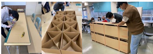
Figure 1. Snapshots of the production of cardboard beds: students (left) cutting a corrugated board paper, (center) fabricating his own cardboard bed, and (right) presenting on his cardboard bed.
