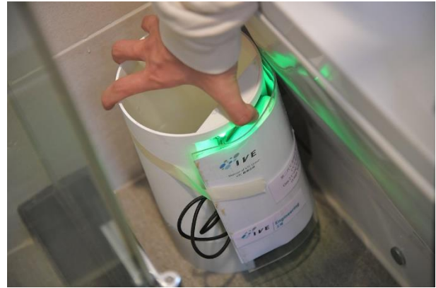
Figure 1: By adding a new attachment to the original design, the upgraded device can be fitted to both floor and wall drains.
