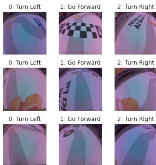
Figure 4 Examples of the custom training dataset for CNN models with a label of either “0: Turn Left,” “1: Go Forward,” or “2: Turn Right.”
