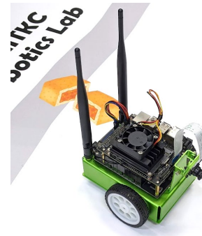
Figure 1 An AI-based robot JetBot used in this laboratory course.
