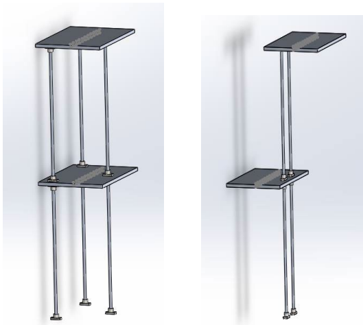
(a) High rigidity (b) Low rigidity Fig.6 Structure of a two-level model
