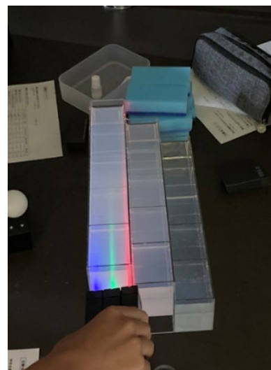
Figure 13: The light of the primary colours transmitting through the solution of wax.
