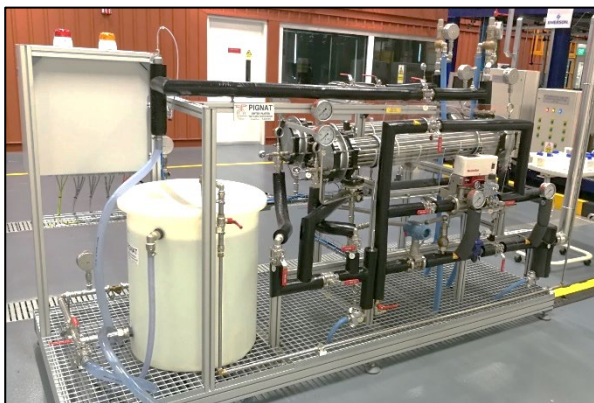
Figure 3. Actual Shell-and-Tube Heat Exchanger Plant
