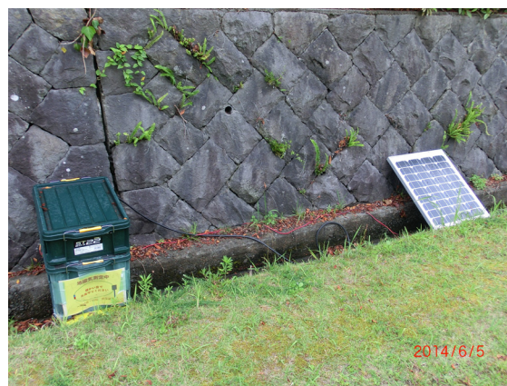
Figure 6 Power system of proton magnetometer.
