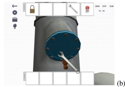
Figure 6, the Fixer apps showing (a)four fault cases, and (b)a user using a spanner to replace a damaged gasket in a water pump to stop water from leaking
