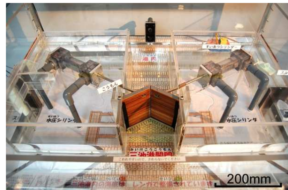
Figure 5 Overview of the Miike port gate technical model
