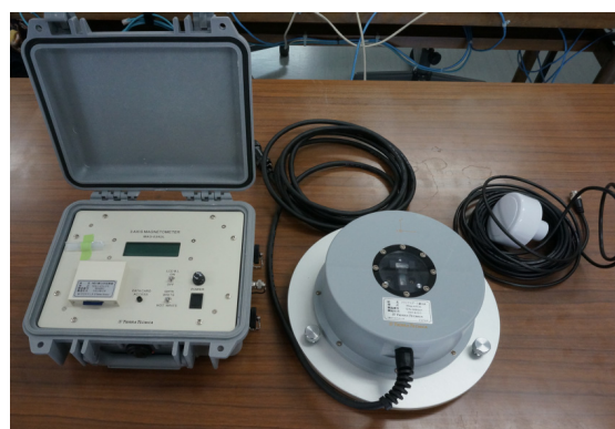
Figure 3 Flux gate magnetometer. The components are an amplifier (and data logger), a sensor, and a GPS antenna (from left).
