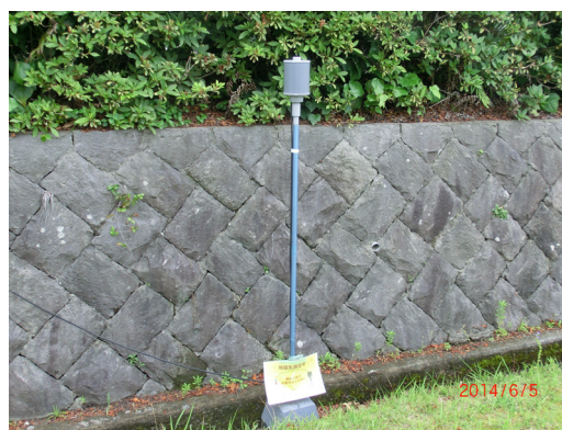
Figure 2 Sensor of a proton magnetometer.
