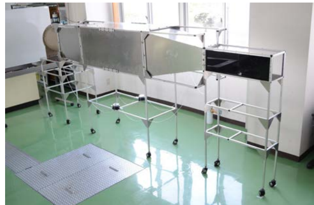
Figure 8 A small wind tunnel for evaluating developed wind turbine.
