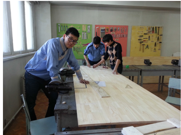
Figure4 measuring the plywood with scale, carpenter's square and pencil.
