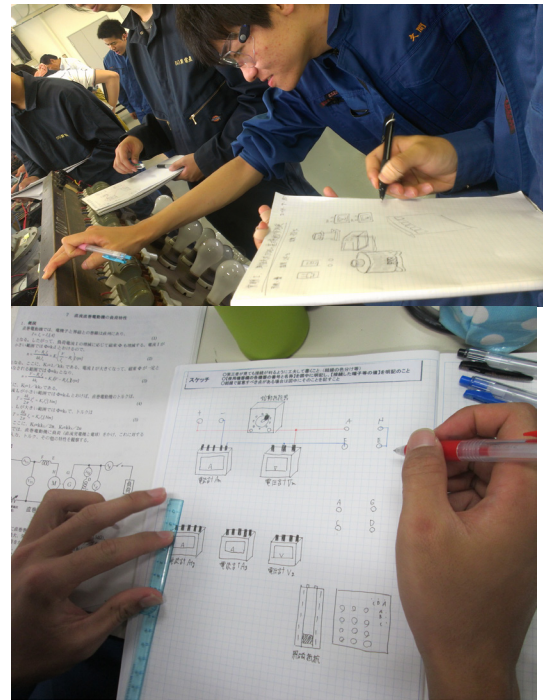
Figure 7 Examples of “Sketch of practical wiring diagram” which written by freehand. (by 4 th grade student at the subject of “Experiments in Electrical Machinery”). Drawing situation (above) and an example of sketch (below).
