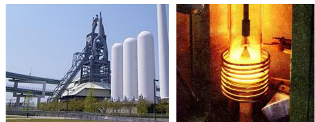
Fig. 4 (a) Yawata Steel Works in Kitakyushu and (b) inductive heating in steel manufacturing.
